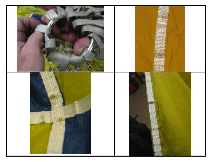
Figure 1: Examples of load tape damage
