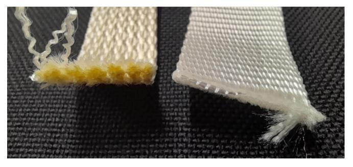
The Polyester Filled Aramid (Kevlar) load tapes (shown on left) is 15 mm wide; the standard polyester tape is 20 mm wide.
