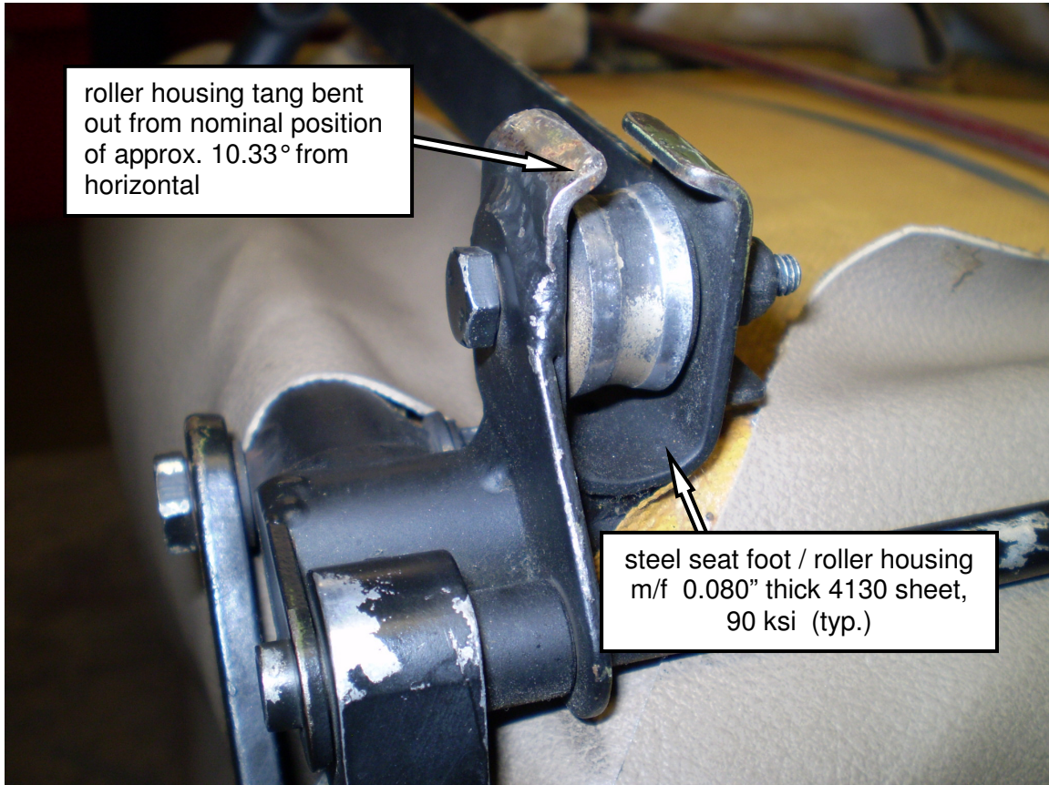
FIGURE 2.0-3 DETAIL OF DEFORMED / BENT SEAT ROLLER HOUSING TANGS
