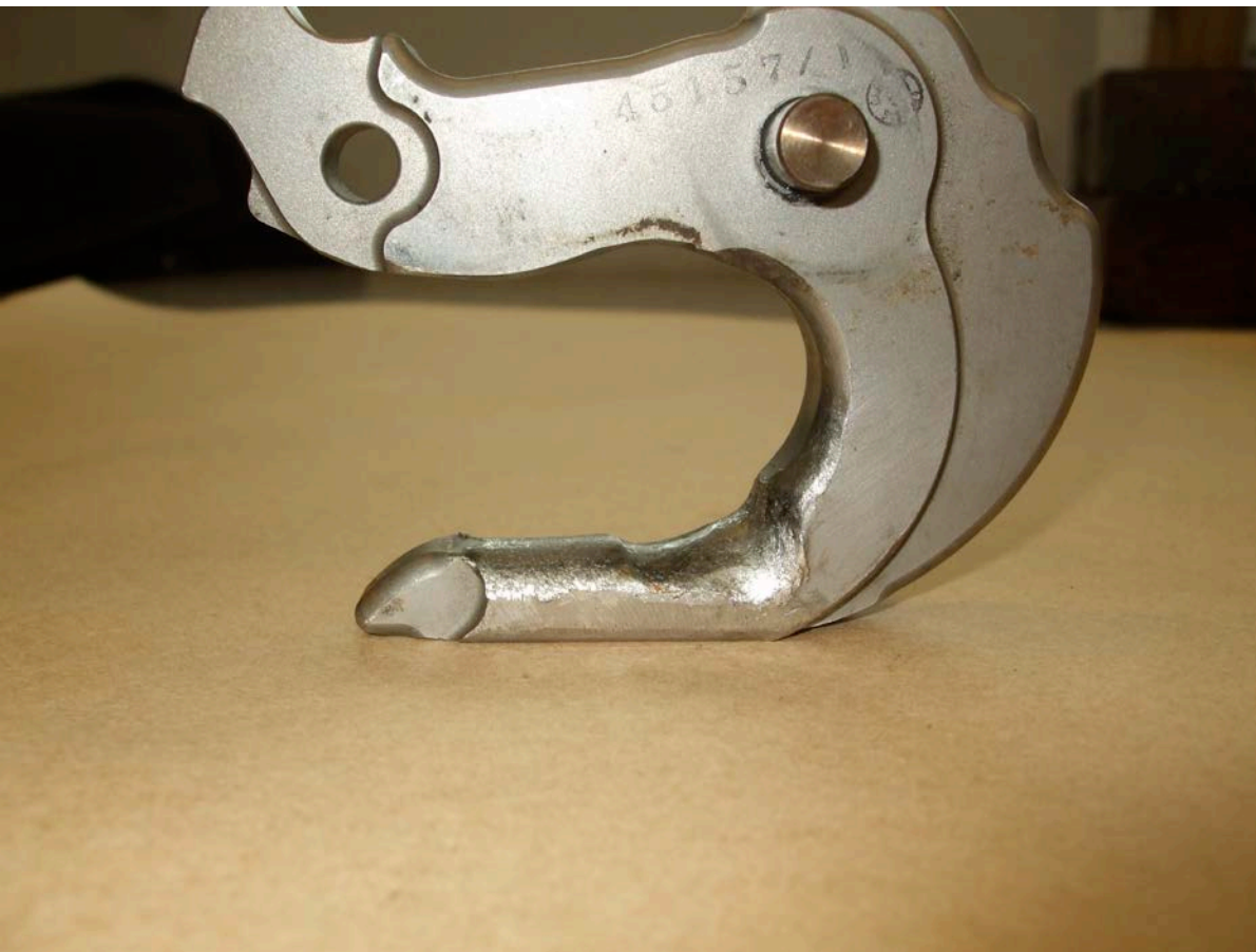
Load beam - Wear beyond manufacturer acceptable limits.
