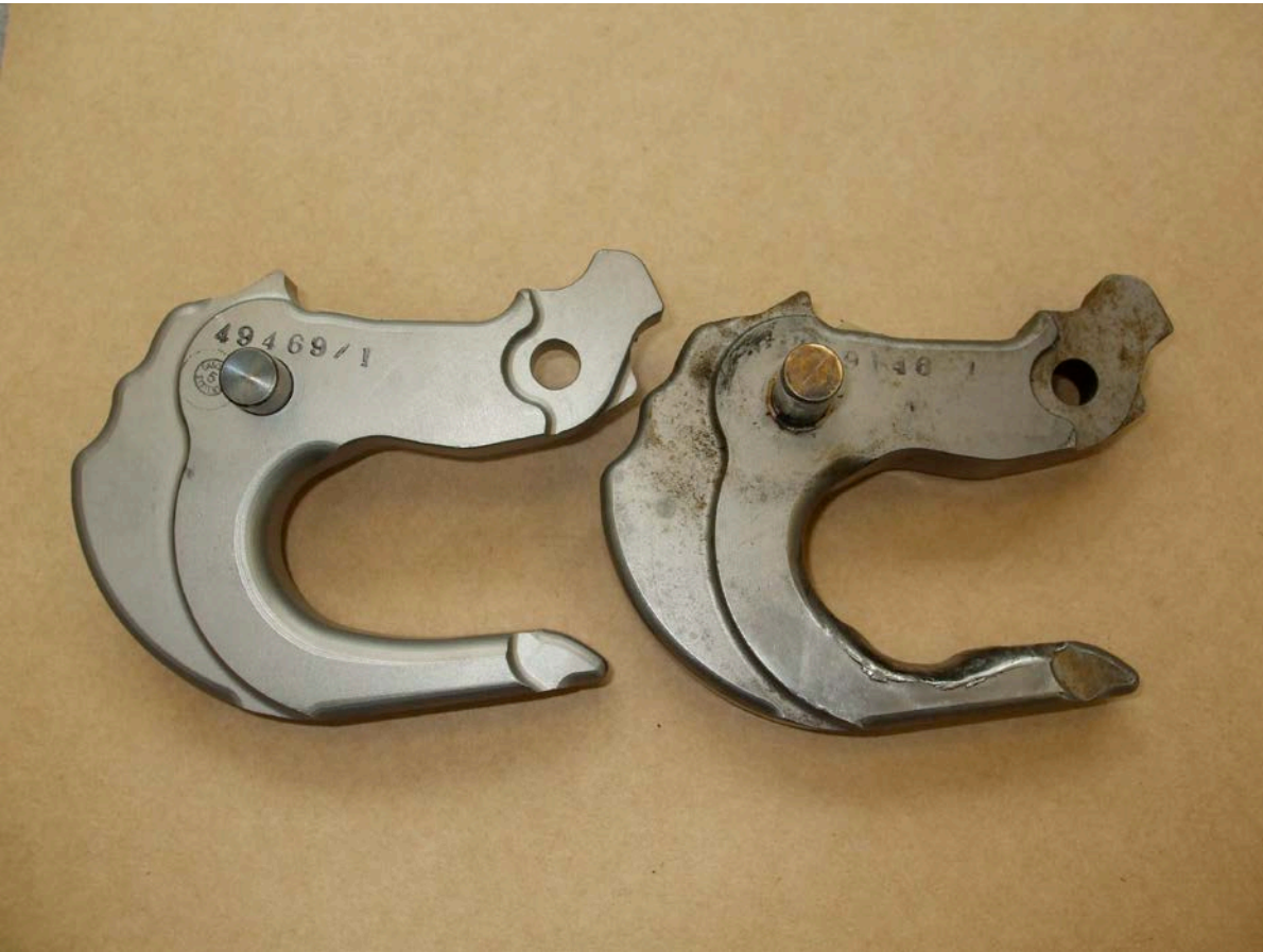
Load beam in the left of the photo – A new replacement part.
