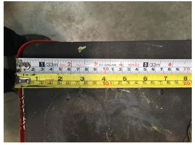
White measuring tape - With a scale marked as 1/33m, which can be mistaken to be 1" increments. Yellow measuring tape - With a correct 1" increment scale.
