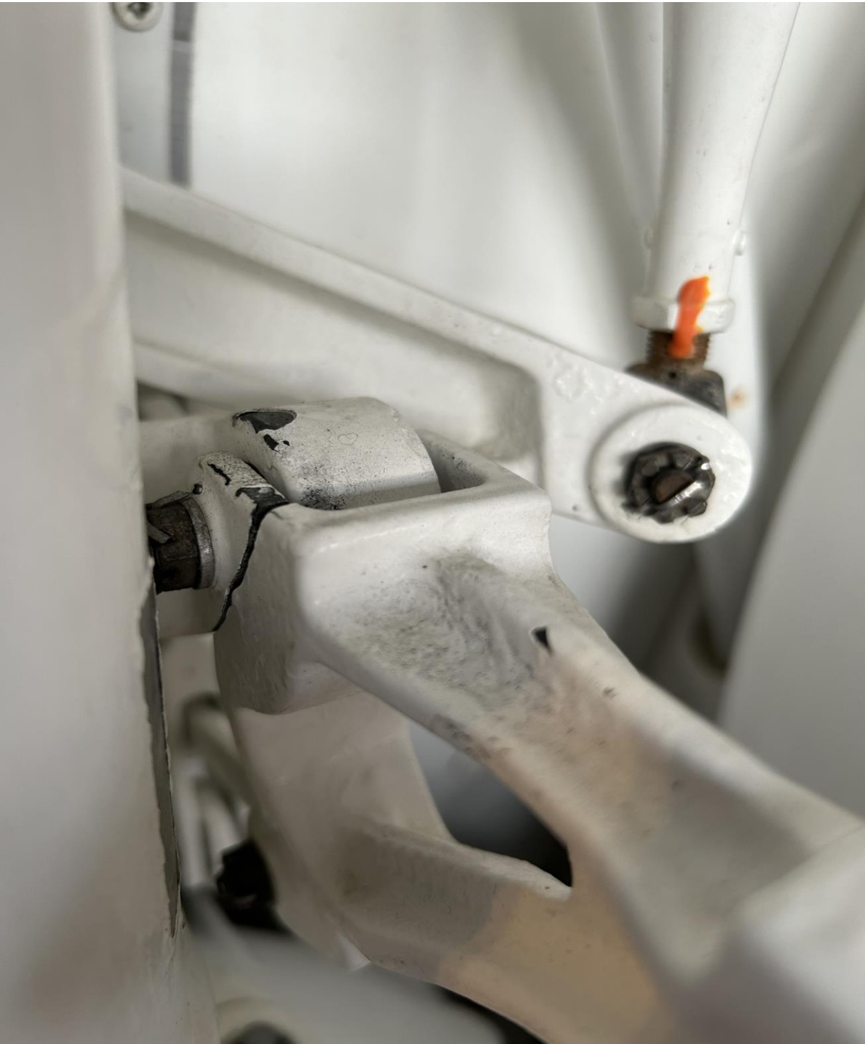
Figure 1 - Cracked longitudinal pitch mixer bellcrank.
