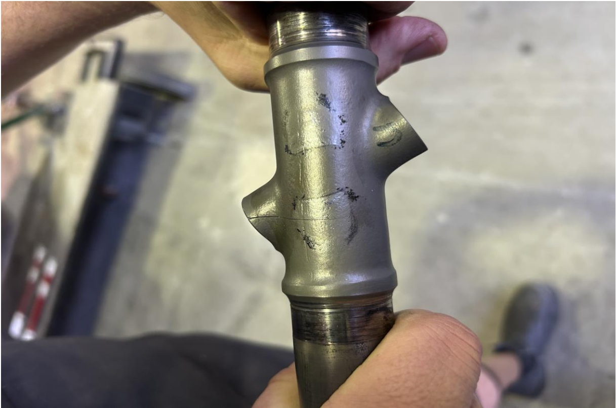
Figure 1 – Hand force applied to exaggerate the crack opening
