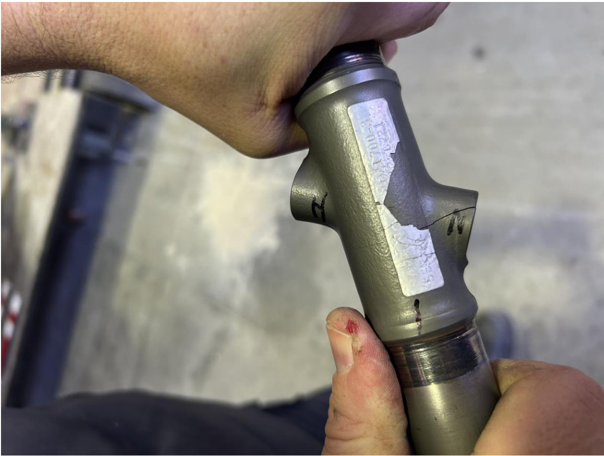
Figure 2 - Hand force applied to exaggerate the crack opening
