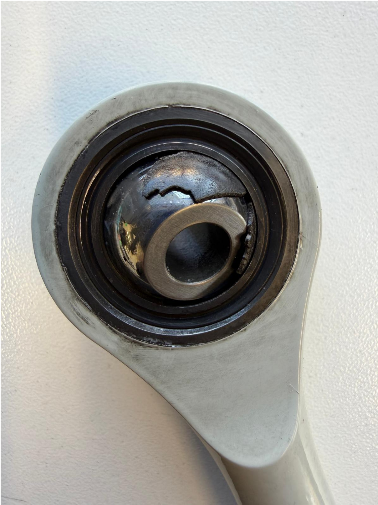
Figure 1 – Extensive bearing liner material damage
