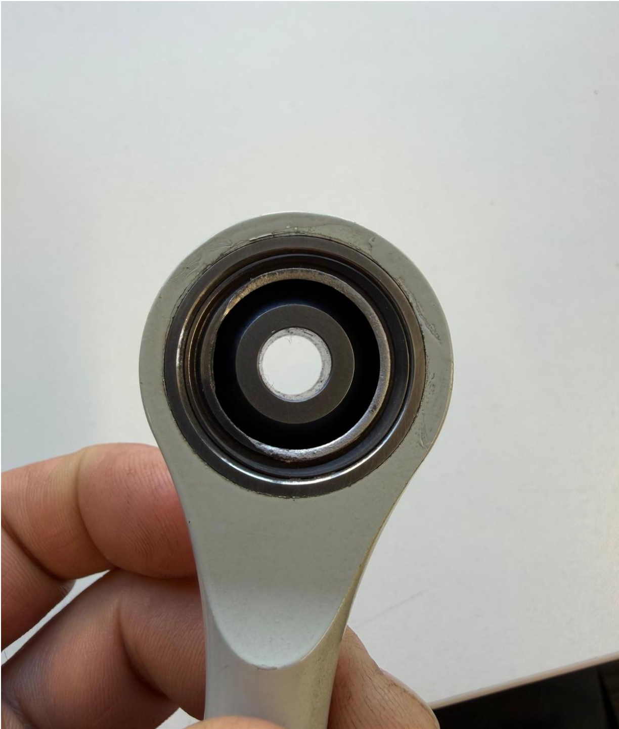
Figure 2 – Complete loss of bearing lining material and resulting damage to surfaces.
