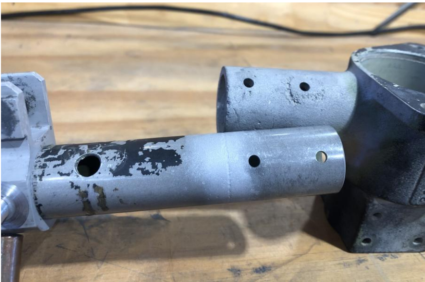
Figure 2 – Collective tube and housing corrosion (paint removed and corrosion partially treated).
