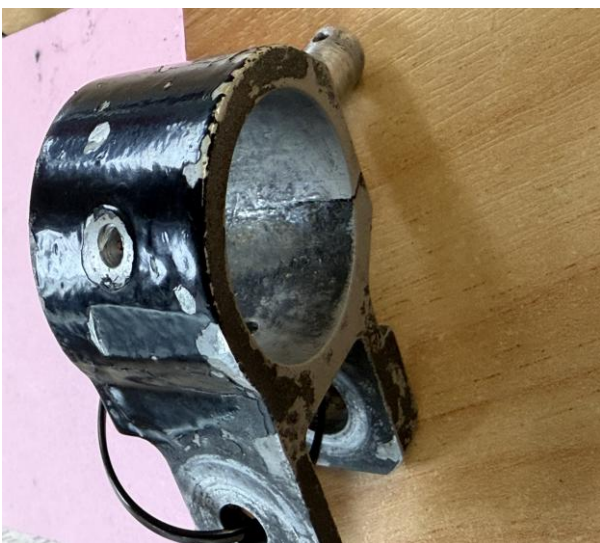
Figure 3 - Collective stick fitting cracking.
