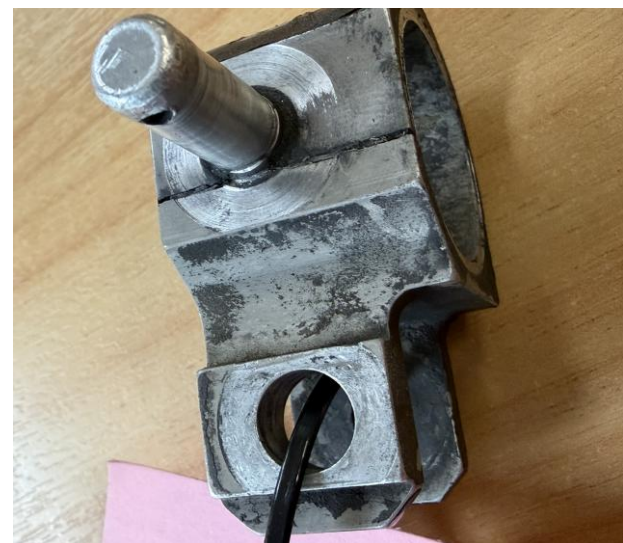
Figure 2 – Collective tube and housing corrosion (paint removed and corrosion partially treated).
