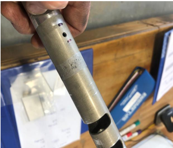
Figure 1 – Collective tube with corrosion and cracking.
