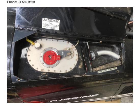
Location of the fuel filler port on the R66 helicopter. (Flush mounted within a flat area under a hinged cowl on the port side of the helicopter).
