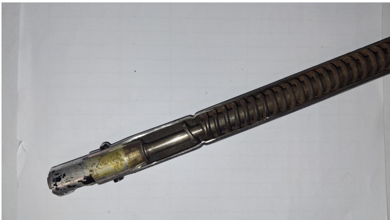
Figure 2 – Failed condition - Washer forced beyond the crimped section of the tube
