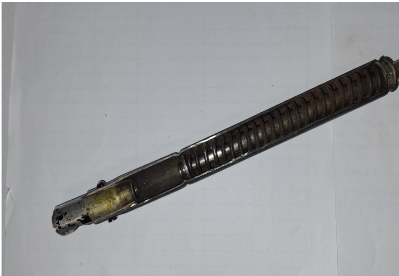
Figure 1 – As intended - washer retained by the tube crimp
