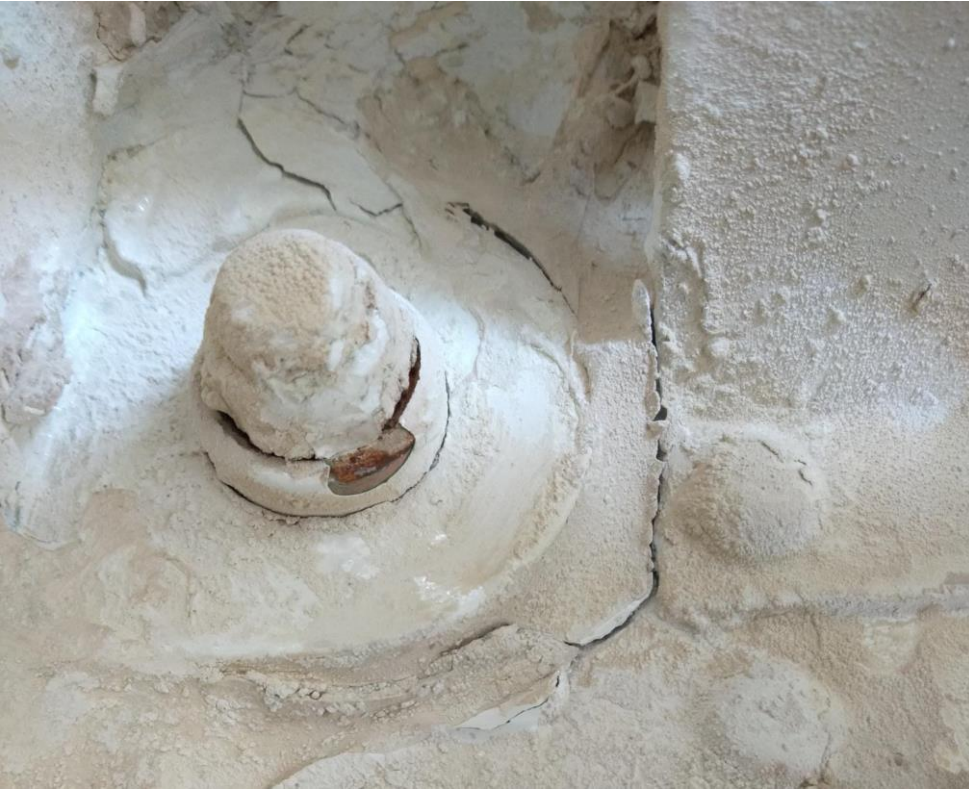
Wing rear spar to fuselage attachment fitting with sealant applied.
