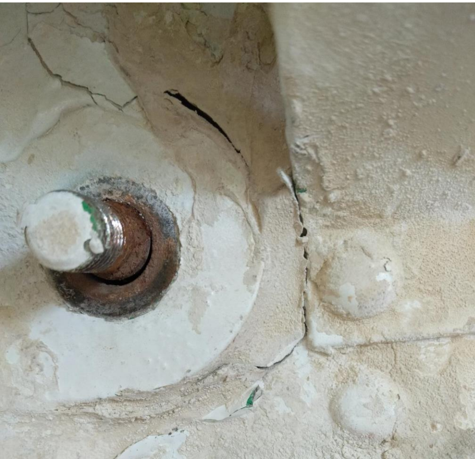
Wing rear spar to fuselage attachment fitting with sealant and nut removed.
