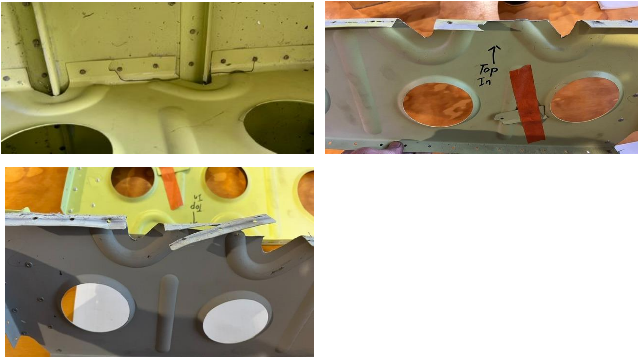
Figure 3 – Rib #2 LH and RH cracking 2 nd aircraft.
