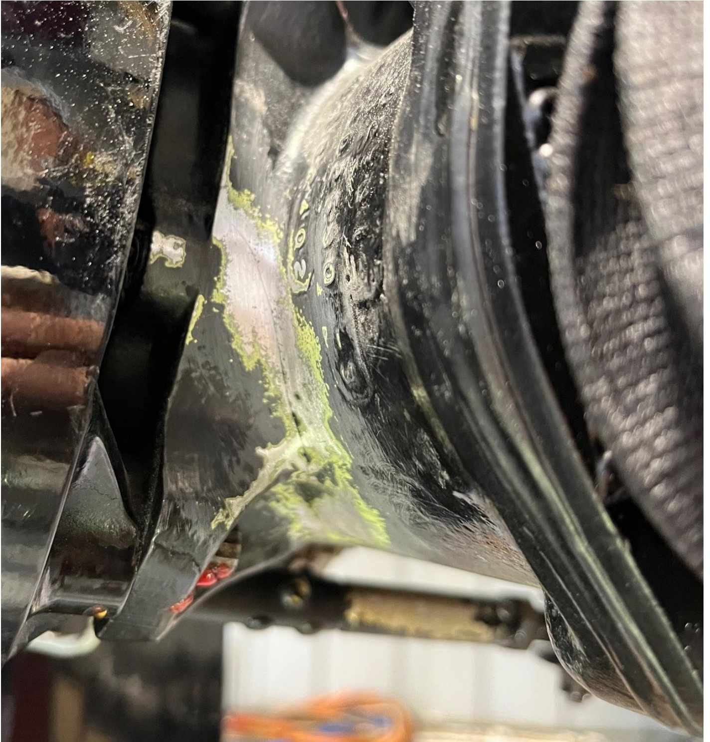
Figure 2 – Crack with paint removed.
