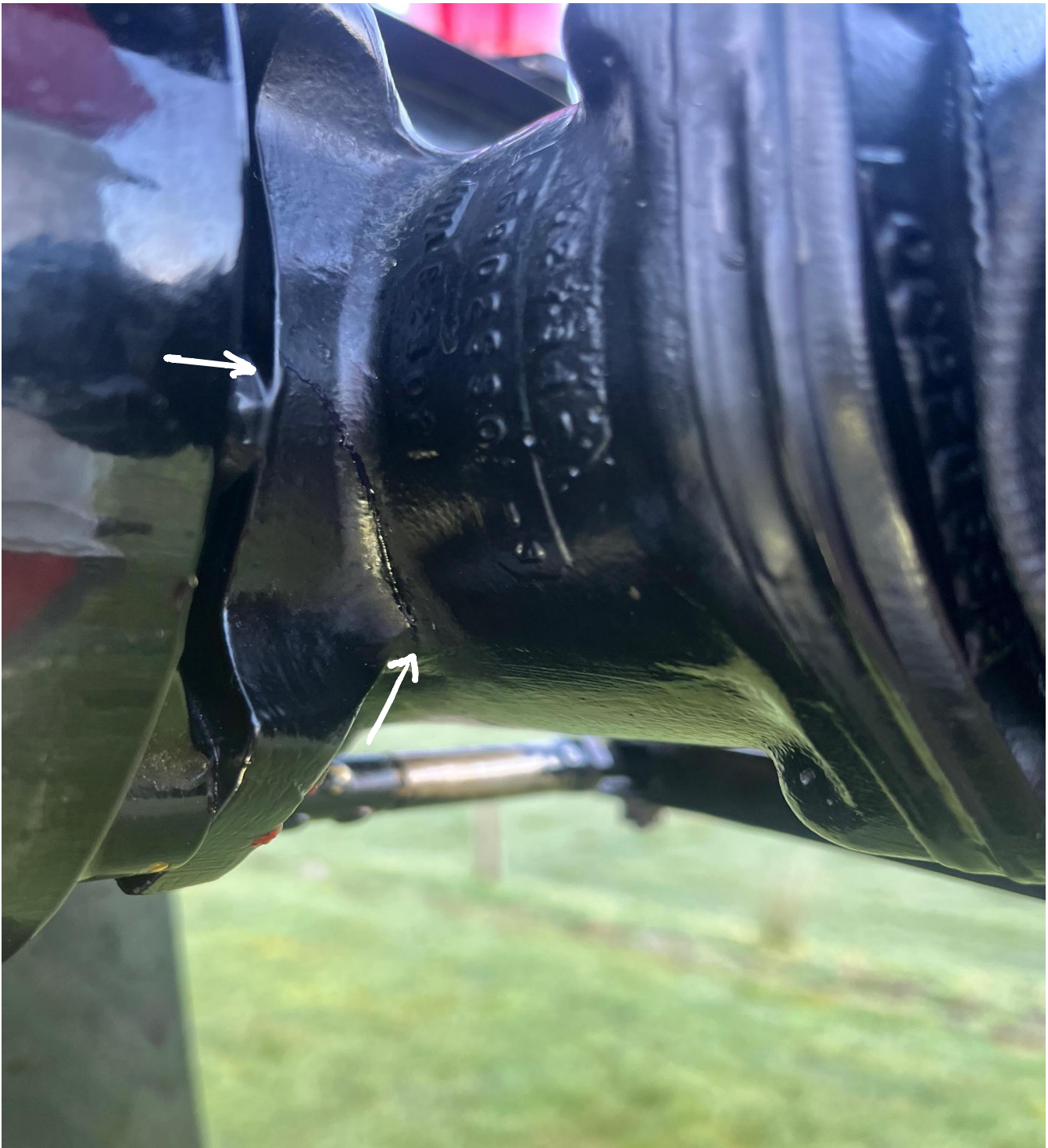
Figure 1 – Tail Rotor Gearbox crack found during the pre-flight inspection. Note the presence of oil residue.
