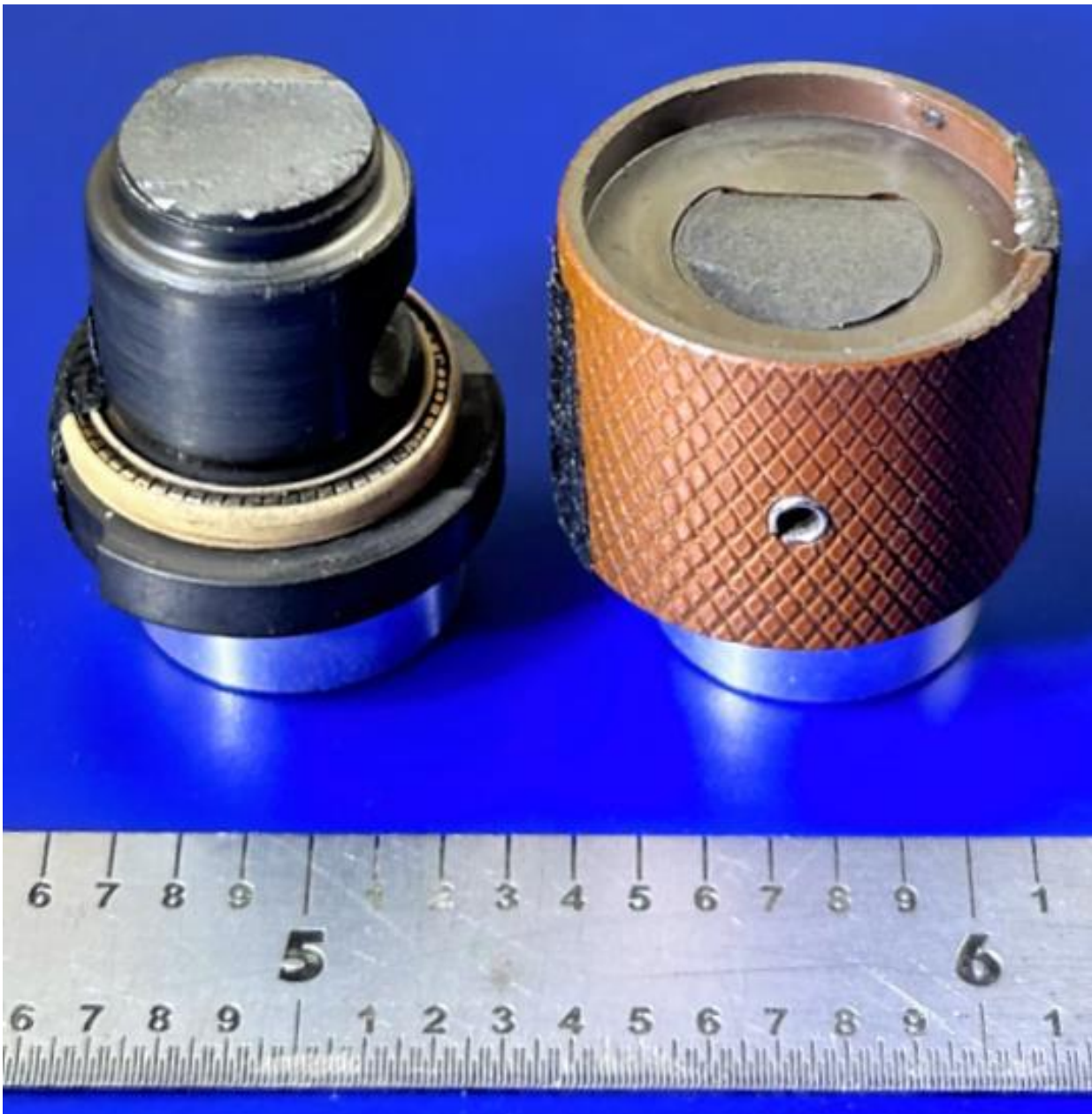
Pc Safety Valve with cracked stem.
