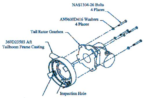
Inspect this area of each bolt. Bolt must protude at least one thread past end of nutplate 4 places.
