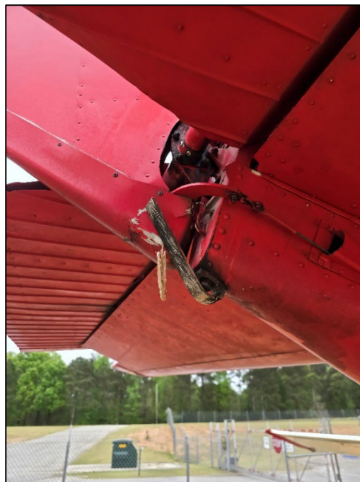
Figure 2. Cessna C172 Tail Skid side view after incident.
