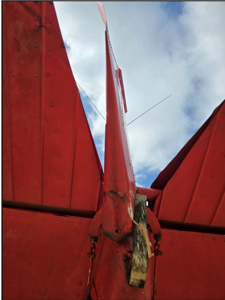
Figure 3. Cessna C172 Tail Skid bottom view after incident.
