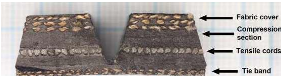
Cross-Section through a v-belt (Revision Z)
