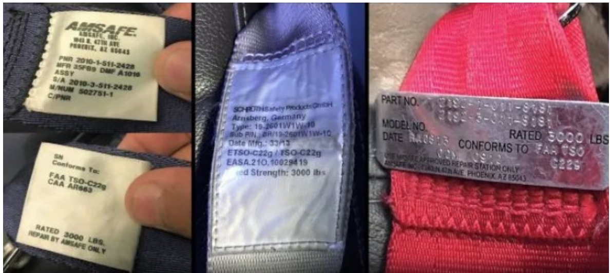
Figure 3 Example label markings of restraints that do meet TSO-C114 or TSO-C22g requirements (Photo credit: AeroSavvy Aviation Insight)
