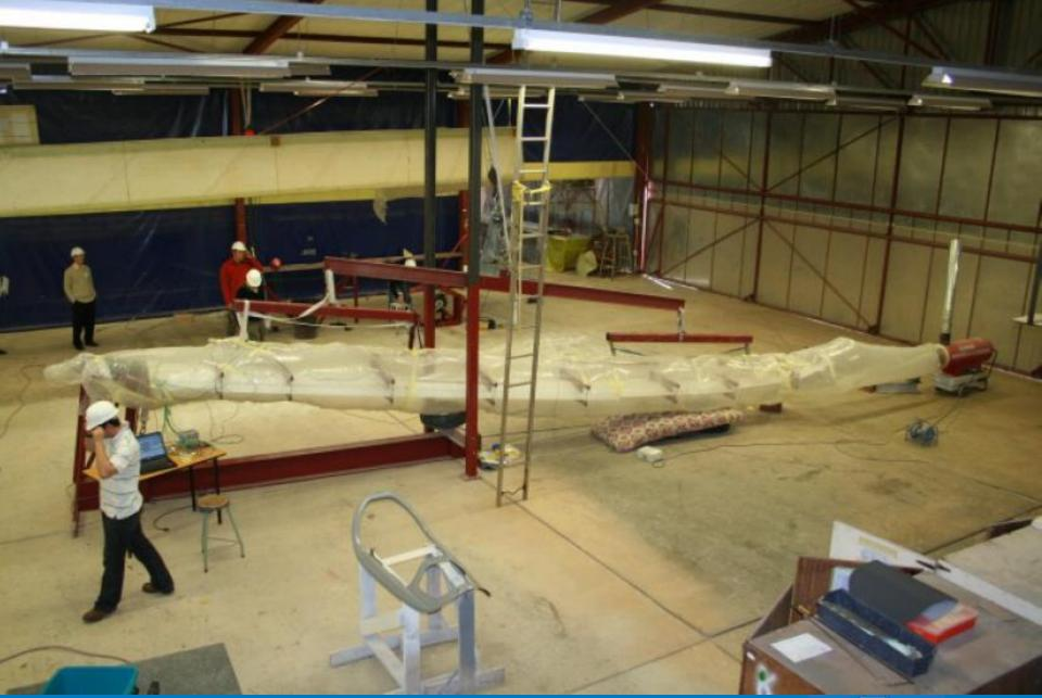
Heat soaked at 57°C for 2.5 hours. Test to be completed within 5 minutes
