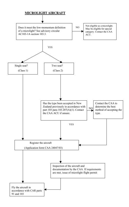
To be eligible as a microlight, all aircraft must meet the definition of a microlight as given in *Advisory Circular AC103-1A*. The definition relates to basic low performance and momentum parameters. If the aircraft does not meet this definition it is not eligible as a microlight (though it may be eligible as a *special category aircraft*). Microlight aircraft are divided into two groups, Class 1 and Class 2.
