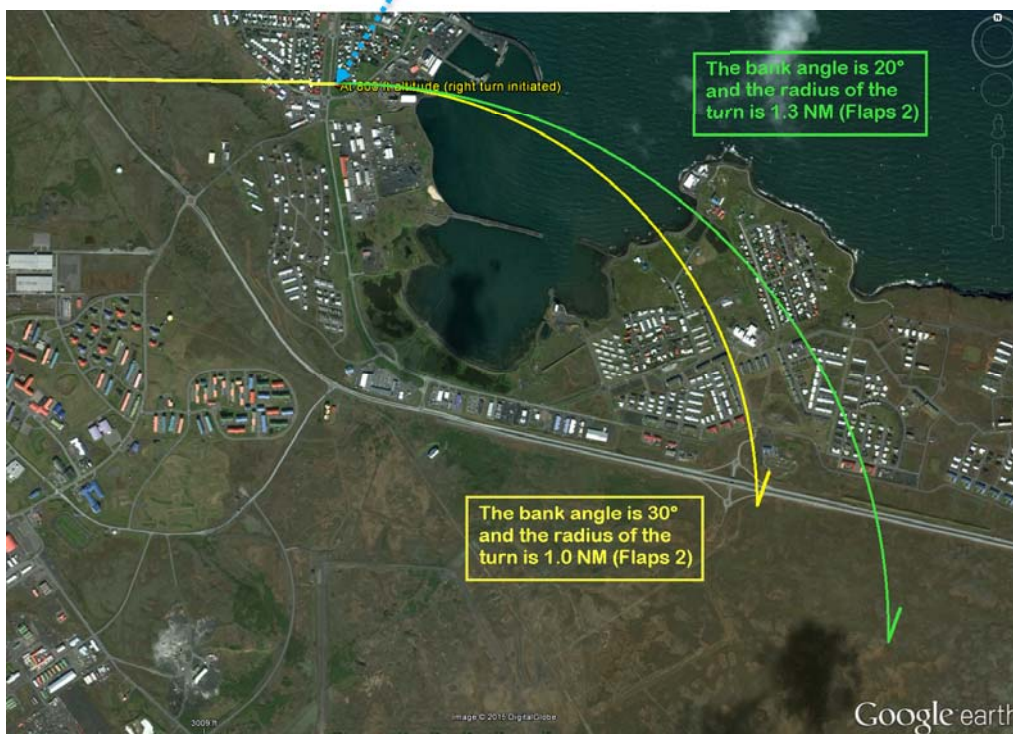
Figure 18: Turn based on right turn at 800 feet altitude for 20° / 30° bank angle
