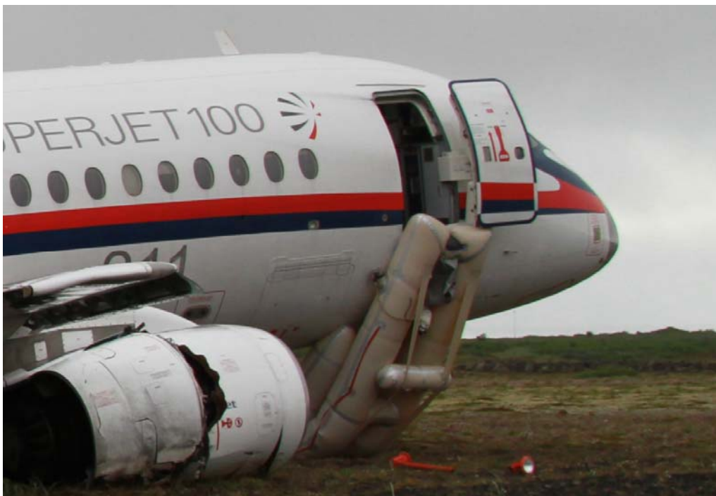
Figure 16: Forward right cabin door slide unusable
