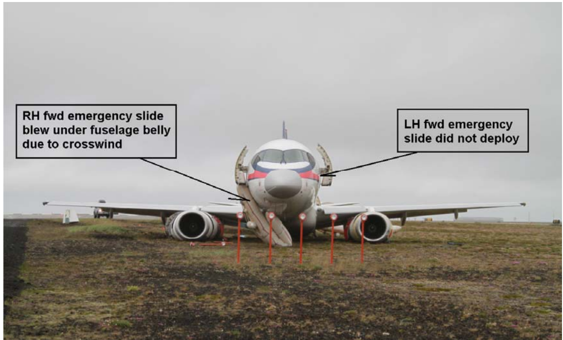
Figure 6: Forward RH emergency escape slide unusable
