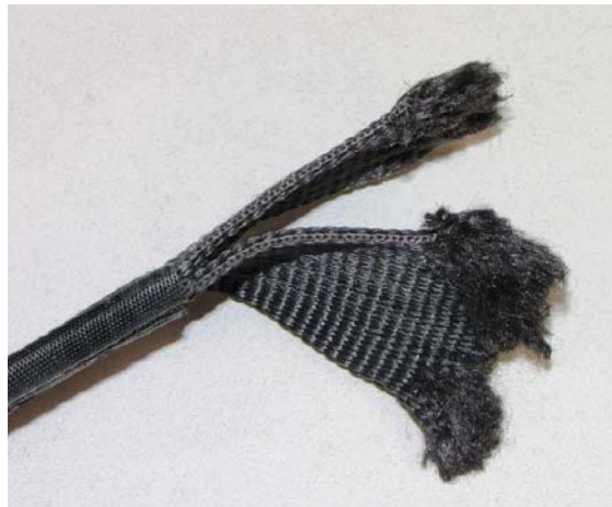
Figure 6: Failed Bridle loop
