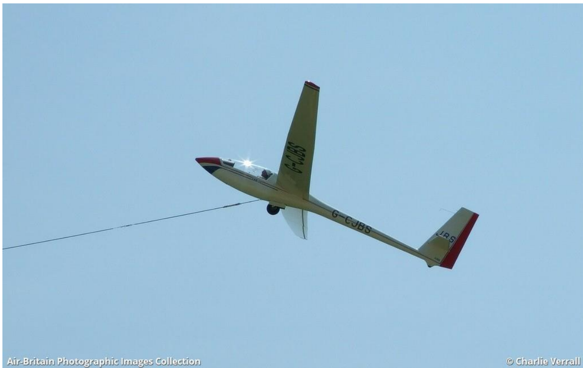
General photo of a LAK-12 under winch launch showing cable weak link - photo with permission of Mr Charlie Verrall
