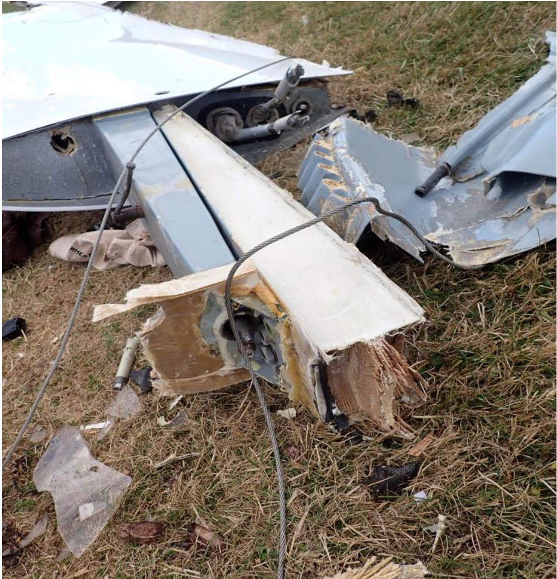
Figure 4. Right wing failure area and wing spar connections pins still in position (fuselage was in the middle section)
