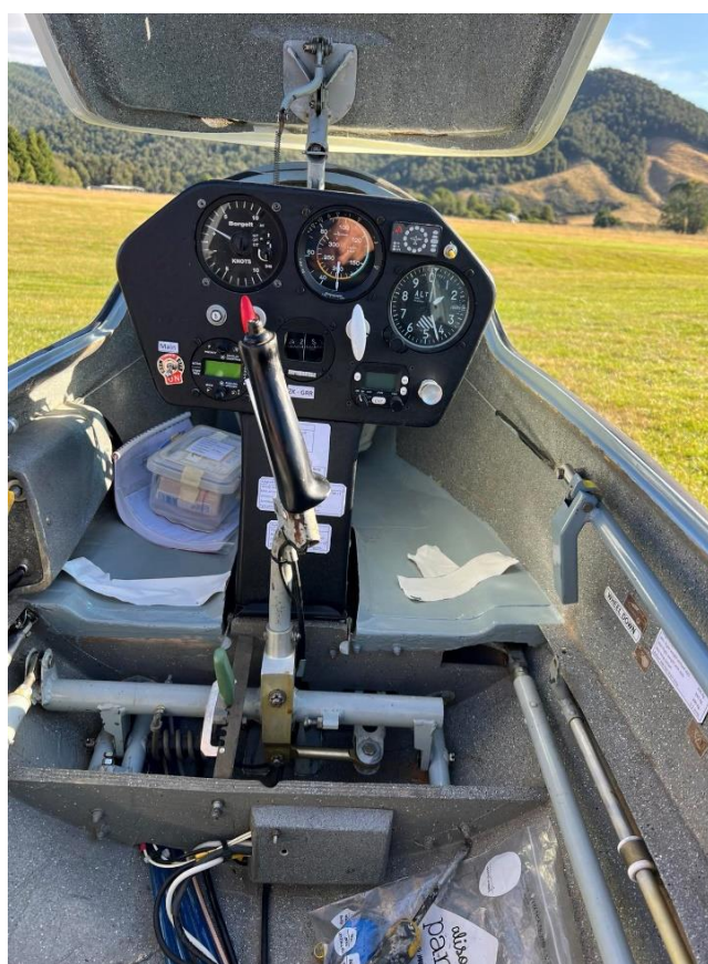
Figure 2. Photo showing GRR left offset control column hand grip.
