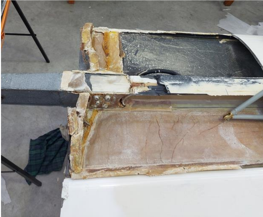
Figure 5. Right-wing failure area (right of four bolts) with spar and wing repositioned for this photo.
