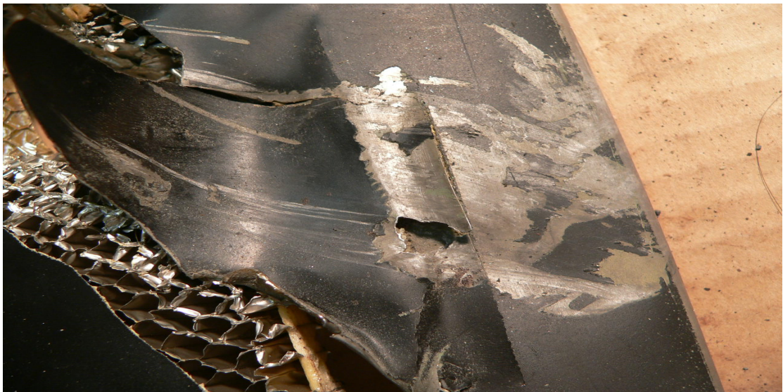
Figure 2 Marks on the main rotor blade caused by contact with the left cabin door.
