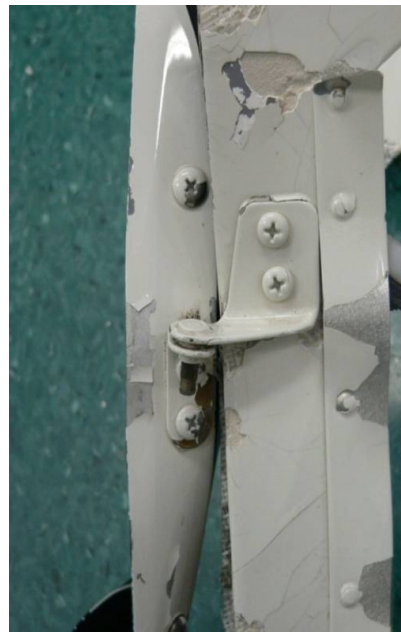
Figure 4 Undamaged lower hinge (reassembled).
