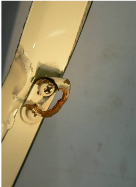
Figure 3 Twisted upper hinge bracket.
