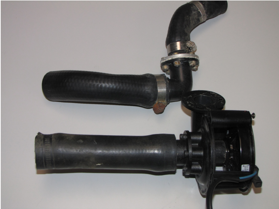
Figure 1, Elbow Tube Arrangement (Top) and Original Auxiliary Coolant Pump (Bottom).
