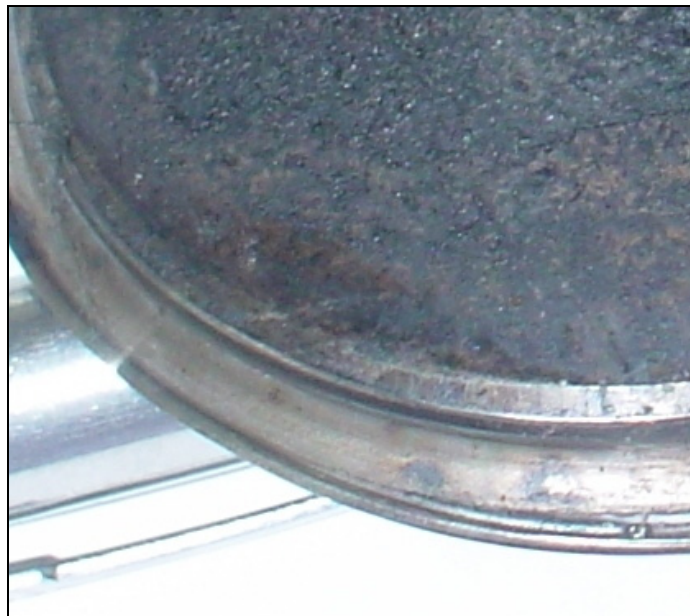
Figure 2: number 5 inlet valve wear
