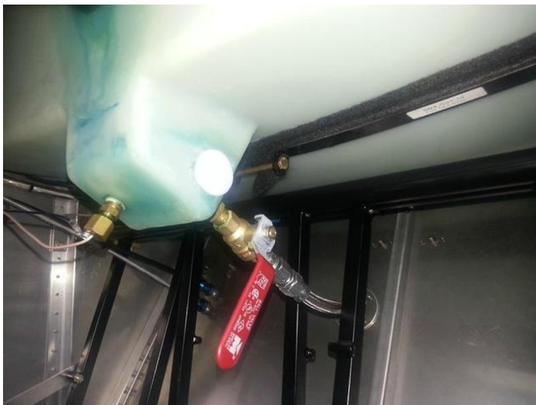
Figure 1. Example of Sonex Waix fuel shut-off valve in the 'off' position. Source: Chris Madsen (2015), accessed May 2023, SonexBuilders.net
