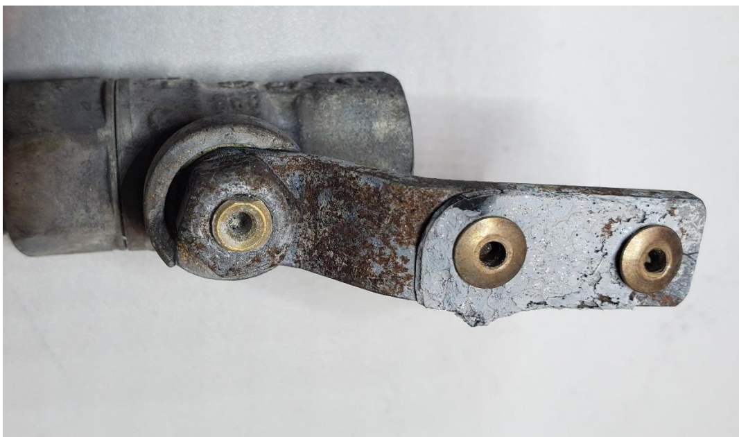
Figure 2. Fuel shut-off valve from ZK-YEX showing remnants of the handle extension, post-accident. (Note the position of the handle in the photograph does not reflect a position pre-impact). Source: CAA photo.
