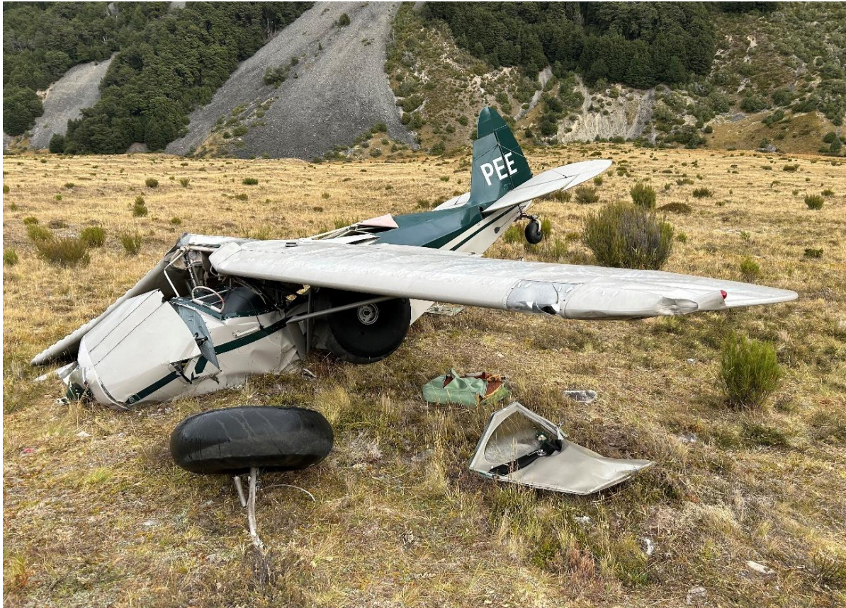
Piper PA-20-135 Pacer, ZK-PEE. S/n 20-962, Dingle Burn valley. The left hand rear cabin door, part of a seat base and a shoulder harness were removed from the aircraft by first responders to aid their access and placed in the locations as seen above. The RH main wheel is in its final resting place and position as found by the people who walked from the airstrip. (CAA photo)
