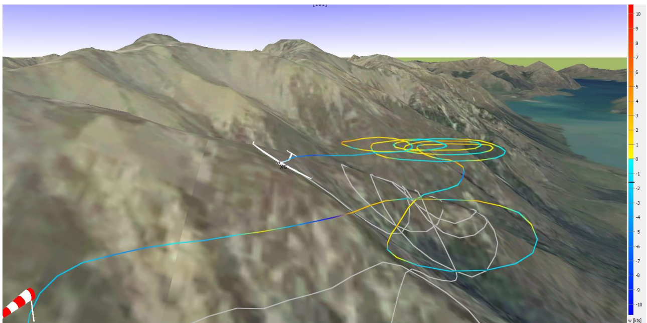
Figure 4: Series of See You™ screenshots of the last 26 seconds of ZK-GXG's flight (Source: GNZ from ZK-GXG LX9000)
