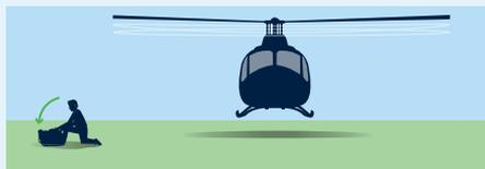
Clear helipad of loose articles. Secure your gear from the effects of rotor wash.
