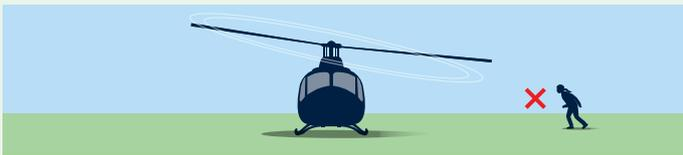
Never approach or leave a helicopter when its engine and rotors are running down or starting up.
