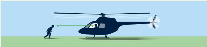
Do not approach without receiving a visual signal from the pilot. Never leave without a visual or spoken instruction to do so. Stay where the pilot can see you at all times.
