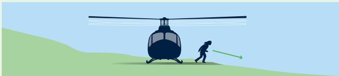
On sloping ground always approach or leave on the downslope side for maximum rotor clearance.
