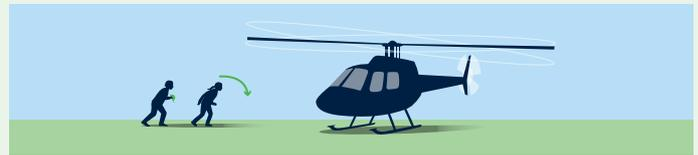
Crouch while walking for extra rotor clearance. Secure any loose articles such as hats and ensure your pockets are zipped up. Never reach up or chase after anything that blows away.
