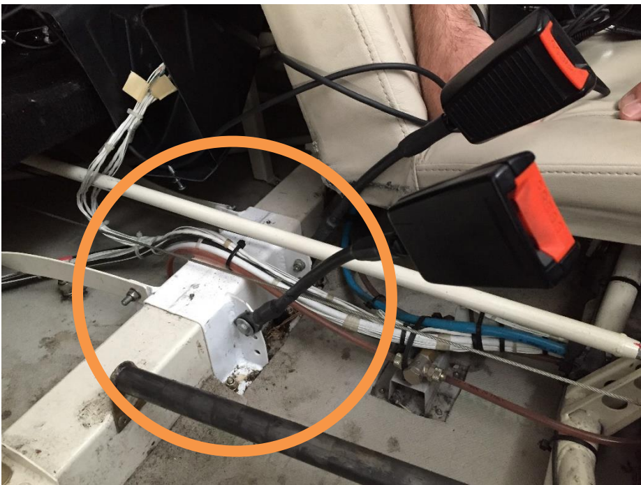
Figure 6: Modified seatbelt anchor point. Seatbelt buckle unable to lift, holding seatbelt more securely across lap.
