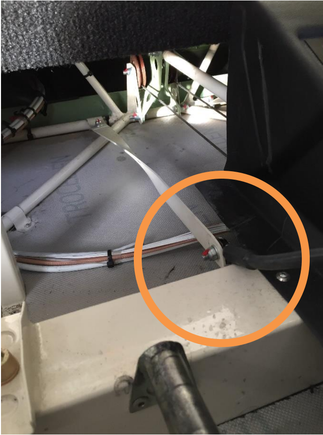
Figure 5: Original Tecnam seatbelt anchor design
