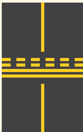
// Runway holding position marking – Pattern A
