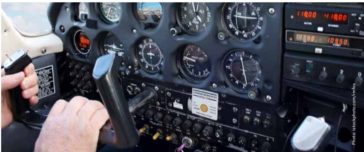
// A view of a cockpit with a carbon monoxide spot detector fitted.
