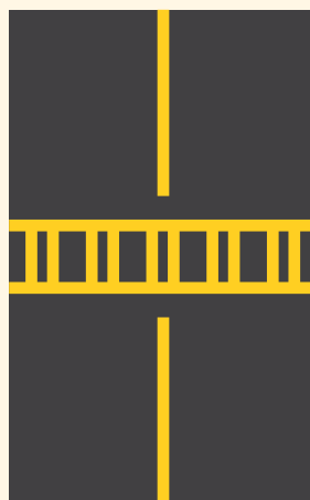
// Runway holding position marking – Pattern B
