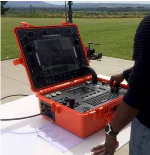
// This photo (used with permission) shows an example of the type of ground control station that will be required for drone operations beyond visual line of site (BVLOS).
