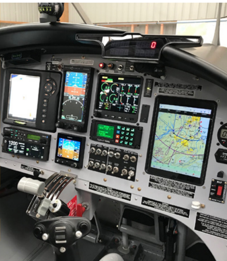
// An example of a NZ CAA-approved STC – an upgrade to the cockpit of an 0800 series Cresco.
