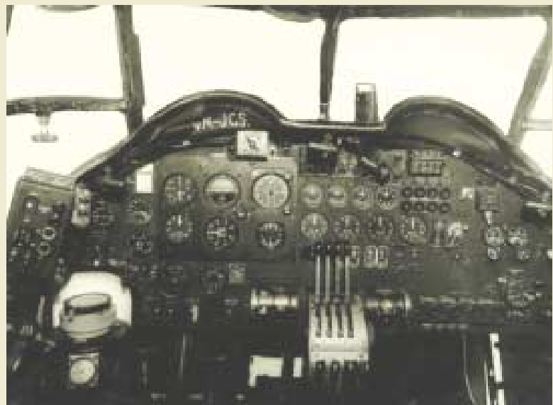
The instrument layout of a Lincoln MK31 that I flew. Sometimes we flew with one pilot and a navigator, who operated the starboard panel. Note the caging knob next to the AH.
