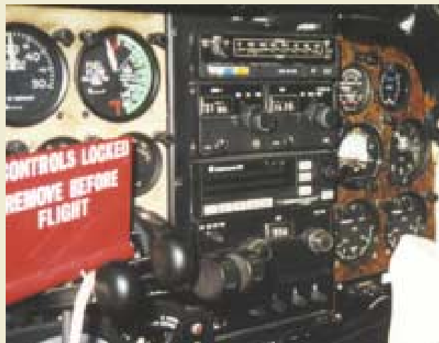
The AH as viewed from the lefthand seat of a Baron B58. The parallax error associated with its position is very apparent; being partially obscured by the radio stack does not help either.
