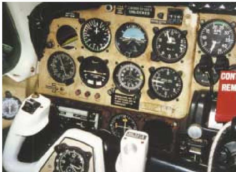
An example of poor cockpit ergonomics. This ILS indicator is positioned low down and behind the control yoke resulting in obstructed vision and parallax error.
