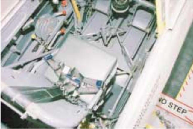
The seat cushion with the straps done up. The straps do not prevent the cushion from moving under negative G.
