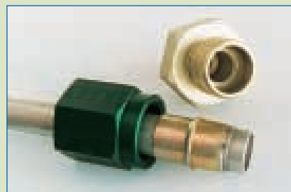
MS flareless fitting components: (Tube, MS 21921 nut, MS 21922 sleeve and MS 21916D reducer)
