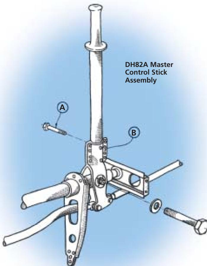
Item 'A' – The missing through-bolt on master control stick.
