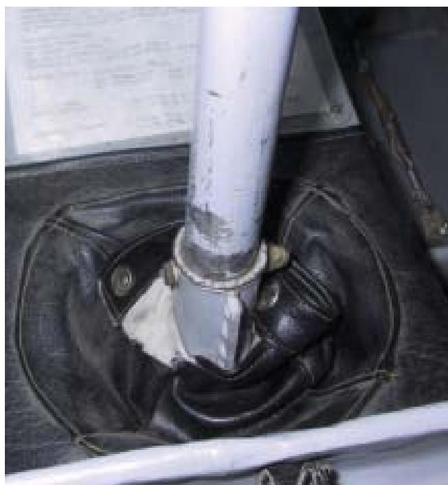
The rear control stick of a DH82A with its attachment assembly exposed.
