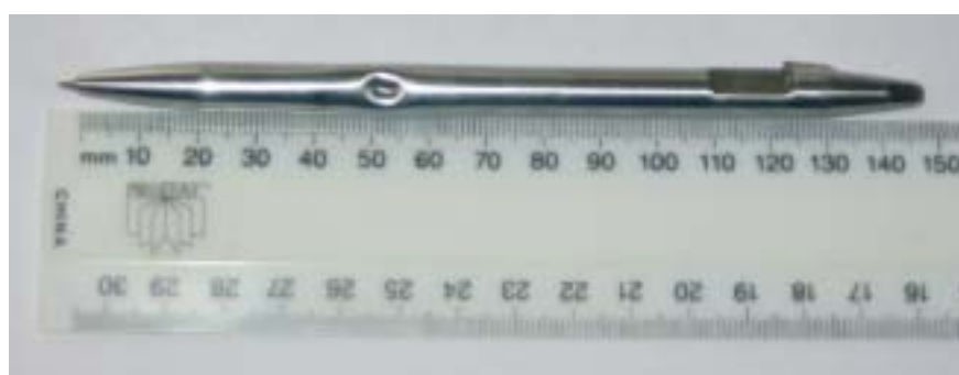
The damage caused by a sprocket tooth.
