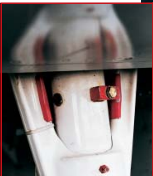
◀ The vertical red turning angle limitation lines and stopper are clearly visible on this Cessna 402 nosegear leg.
