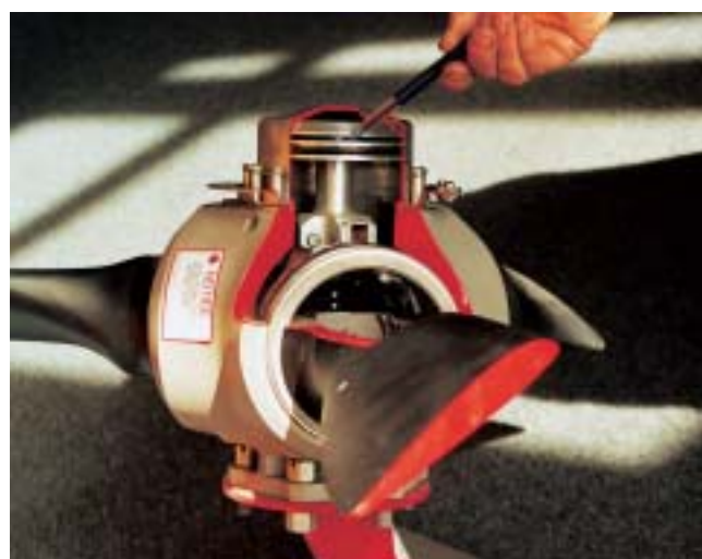
A cut-away of a McCauley C200-C400 threadless propeller showing the fine-pitch stop. Adjustment requires specialised tools and oil draining and is normally an overhaul shop task.
