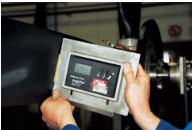
The blade angle being measured at the manufacturer's reference station, which is normally a specified distance from the propeller hub centreline.
