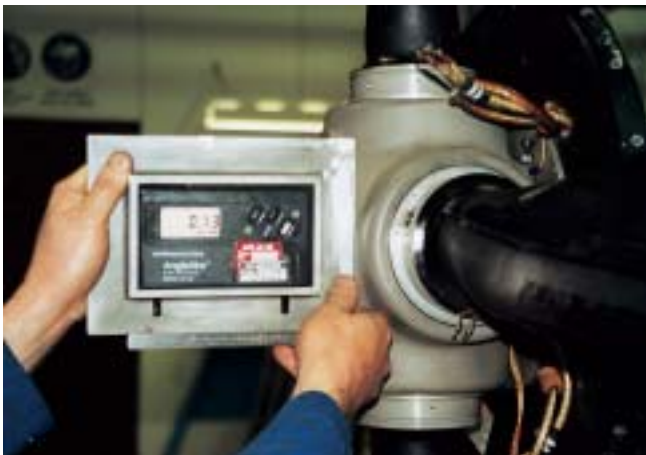
Obtaining the propeller reference plane before measuring the blade angle.
