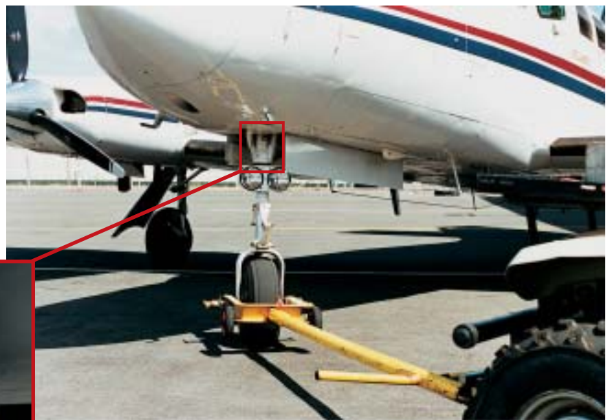
◀ The vertical red turning angle limitation lines and stopper are clearly visible on this Cessna 402 nosegear leg.
