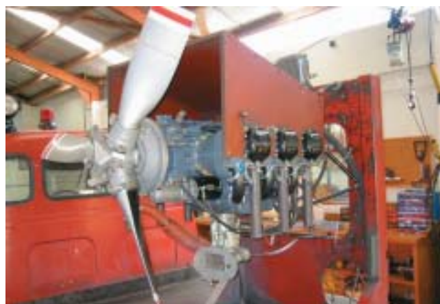
A Lycoming O-540 fitted with a test club propeller on the test stand.
