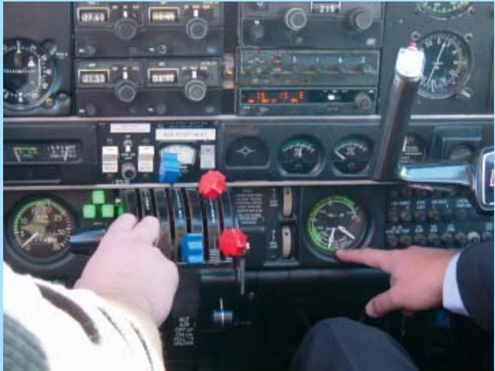
thinking that they were in fact the fuel pumps, the consequences of which did not become apparent until the loss of manifold pressure was noted. In the meantime, the student had also turned the lefthand engine magneto switches off confusing them with the landing light switches as the last item on the checklist. (The magneto switches are located directly above the landing light switches and have a cover over them to prevent them being inadvertently selected, which the student lifted.)
