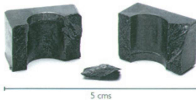
The New Zealand agents for the propeller, Aeromotive Ltd of Hamilton, quickly found the problem. A small plastic spacer in the hub had fractured, due, they believe, to a lack of grease. The problem of grease escaping from those hubs was well known. The manufacturer, MT Propeller of Germany, had previously issued two engineering changes to alleviate the problem, with little success. They have now
