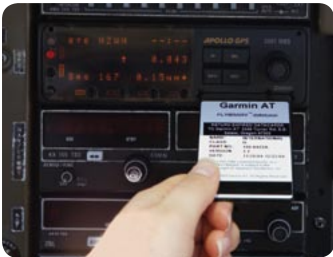
Regardless of the GPS database source, cross-check against a hard copy of enroute or area charts, and approach plate tracks and distances, before departure.
