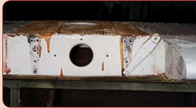
Further inspection on the tailplane revealed that the starboard mounting bracket (on the left in this photograph) had shorn off completely, and that the port mounting bracket was ‘holding on’ by one attachment rivet.
