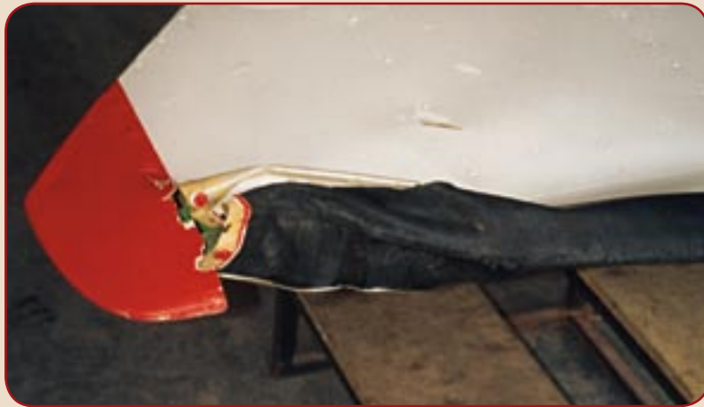
Damaged tailplane from the agricultural aircraft.
