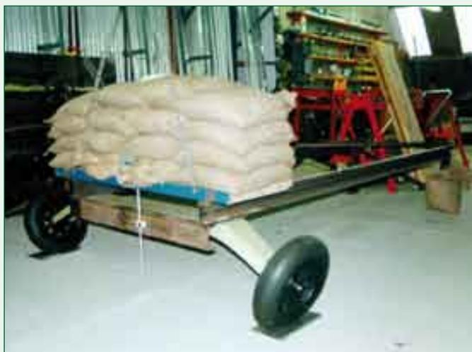
Undercarriage 'drop testing' is part of the certification process. The undercarriage of the Bantam B22J is constructed of fibreglass.
