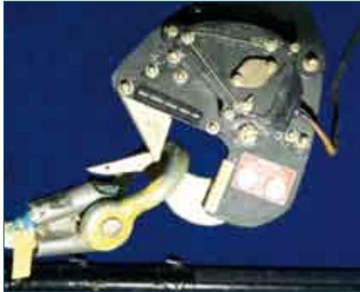
tension. This means that it may be difficult or impossible to jettison a load in an emergency, or the pilot may find that the load is still firmly attached to the hook even though the release mechanism has been operated.
