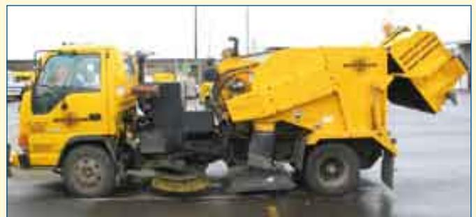
Building stands were swept on a random basis. Now every available stand, remote stand, and the inner pier road are swept every night, together with 'hotspots' identified by airfield staff on a daily basis. The driver holds a Stage 2 Airside Driving Permit meaning the vehicle can be driven on the movement area.
