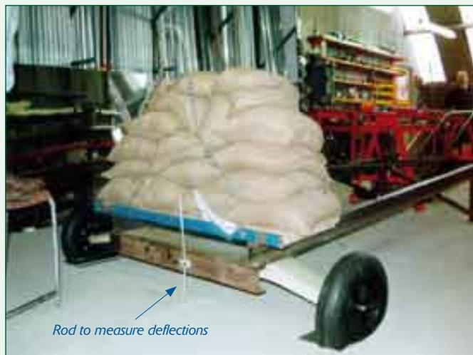
A test weight of 450 kg is dropped from a height of 224 mm to simulate load forces on the undercarriage.
