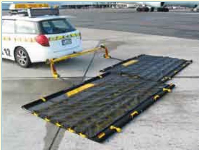
The 'Boss' was used extensively in the final stage of the four-year runway rehabilitation. The outboard engines of large aircraft were blowing loose material onto the taxiways, but two or three runs with the 'Boss' picked everything up.
