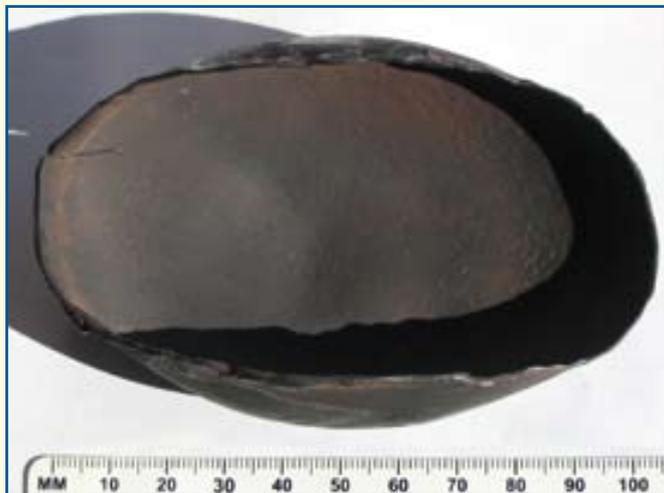
In the absence of an aircraft turning up with a piece of its exhaust obviously missing, theories about it being an internal component blown out had to be considered. The object is 6.5 cm wide at the widest point, which means that any exhaust outlet would need to be wider to eject the component.
