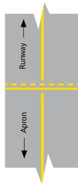
In some domestic aerodromes in New Zealand the holding position marking may still be a single line with a dashed line closest to the runway.
