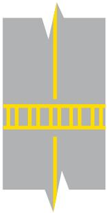
**Pattern 'B'** runway holding position marking is used to identify a holding point further away from a runway than a pattern 'A' runway holding position marking. A pattern 'B' runway holding position marking has two lines across the runway that are intersected at 90 degrees by small lines. It looks similar to a ladder across the taxiway.
