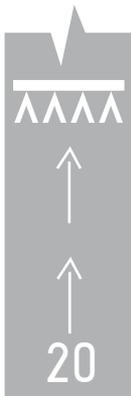
Temporarily Displaced Threshold
