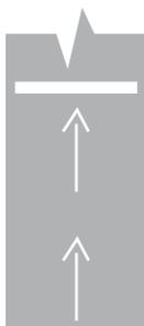
Permanently Displaced Threshold
