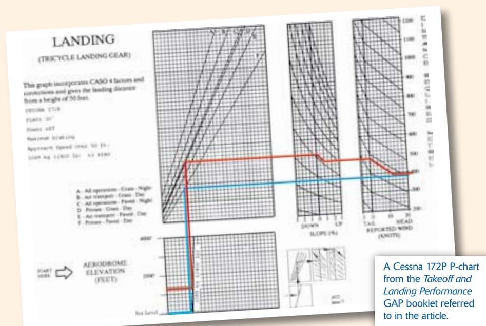
Once a chart has been created, it is a quick and convenient method of establishing runway length requirements.
