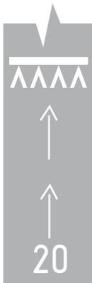
Temporarily Displaced Threshold
