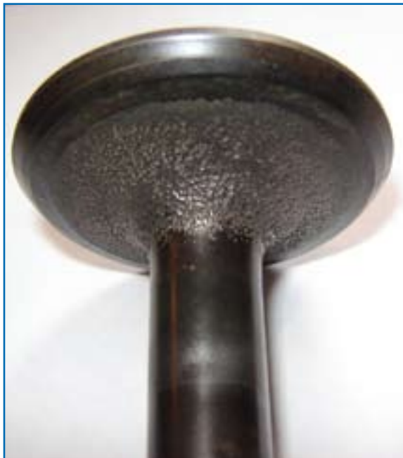
This exhaust valve has only been in service for 19 hours and shows severe damage caused by over leaning. Failure at the neck of the stem would eventually result. Picture courtesy of Lycoming A Textron Company.
