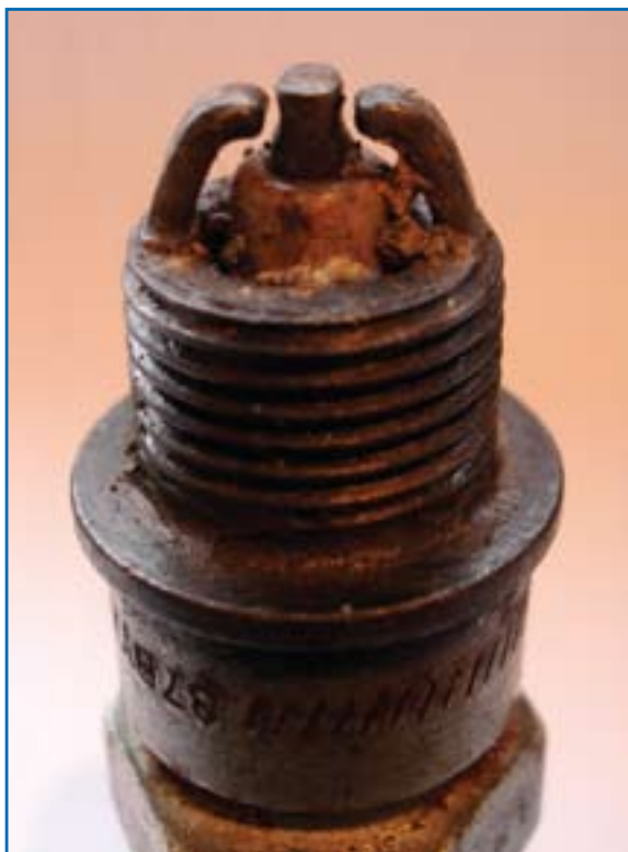
Cessna 152 – Lead fouled spark plug.
