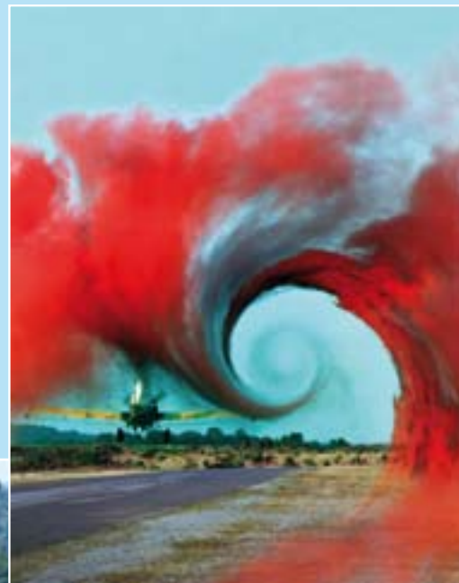
▲ Wake vortices generated behind a light agricultural aircraft (Thrush Commander) in a wake vortex study conducted by NASA. Photo courtesy of NASA Langley Research Center.
