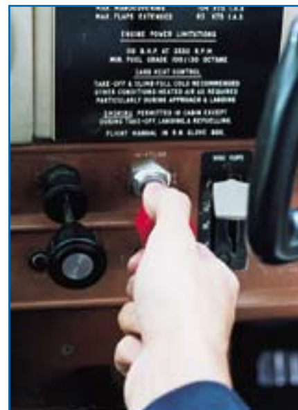
When leaning, adjust the mixture lever slowly.
