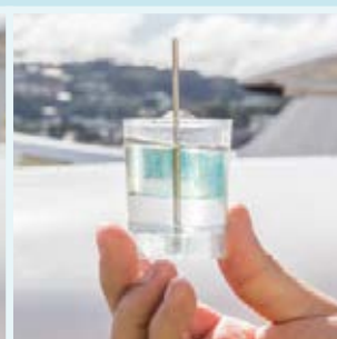
Mix of water and fuel
