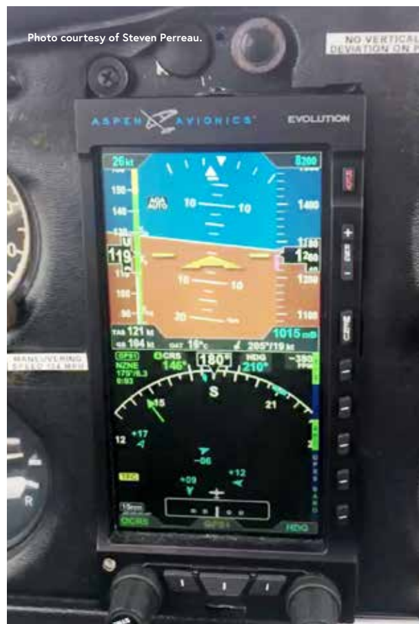
// Aspen showing live ADS-B in traffic displayed in ARC mode in flight.
