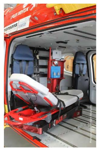
// This Flight Structures system in the new Auckland Rescue Helicopter Trust AW 169 has the stretcher in the transverse position for loading the patient, but then swivelling to the longitudinal position for flight. That allows the medical team substantially more room to work on the patient, including stabilising them during flight, rather than on the ground. That could save up to 30 minutes in delivery to the hospital.
