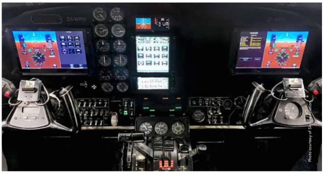
// Skyline Aviation in Hawkes Bay carried out an electrical load analysis when it upgraded its King Air B200 with a Garmin G600 TXI Avionics suite.
