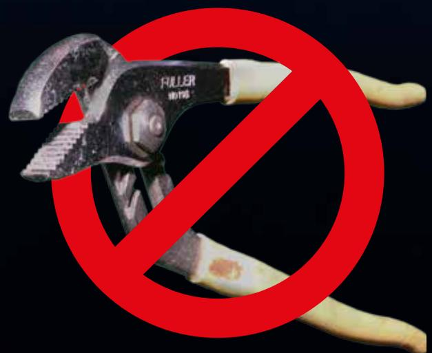
Multi-grip or poly grip pliers shouldn't be used anywhere on any aircraft. They can damage the fitting too easily.
