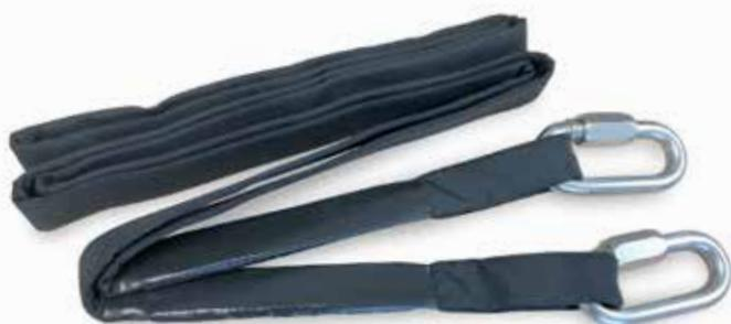
If activated, this could have resulted in the rocket launching and pulling the Kevlar strap through the incorrectly fitted carabiner, therefore not deploying the parachute.
